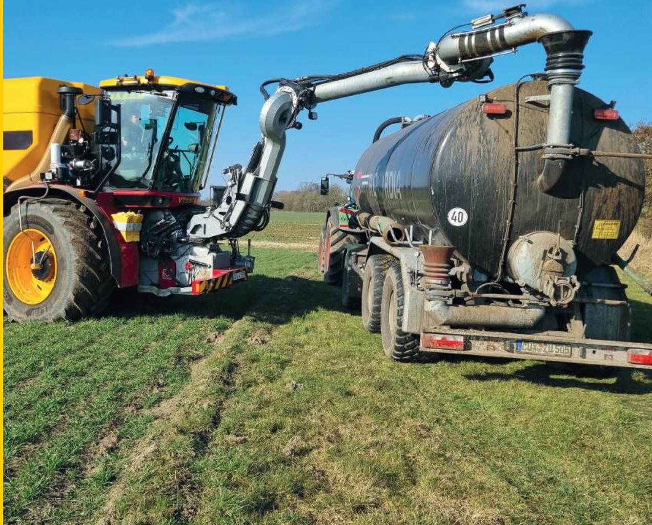
The VT5536 comes with a multifunctional suction arm as standard at the front of the machine. Thanks to our unique design, the suction arm has 160° movement, which means that it can be used, both at the side and the front of the machine. In every position, the driver has an unhindered view of the arm without having to look back.
