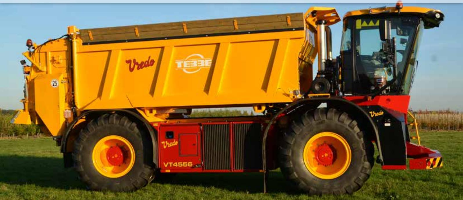
Beside the Vredo VT4556 in slurry application, Vredo developed a version for spreading solid fertilising materials over the fields. This can be manure, but also compost, lime, sludge or sewage cake. The characters of the solid fertilizers have many variables and give a lot of possibilities in relation to the:
